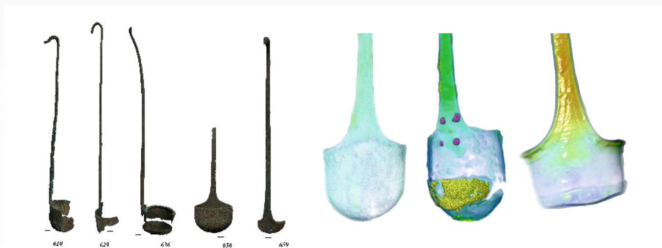
Photo of several samples under study and reconstructed 3D models with highlighted elements of the construction of ancient bronze kyathes based on neutron tomography (NRT, IBR-2).
