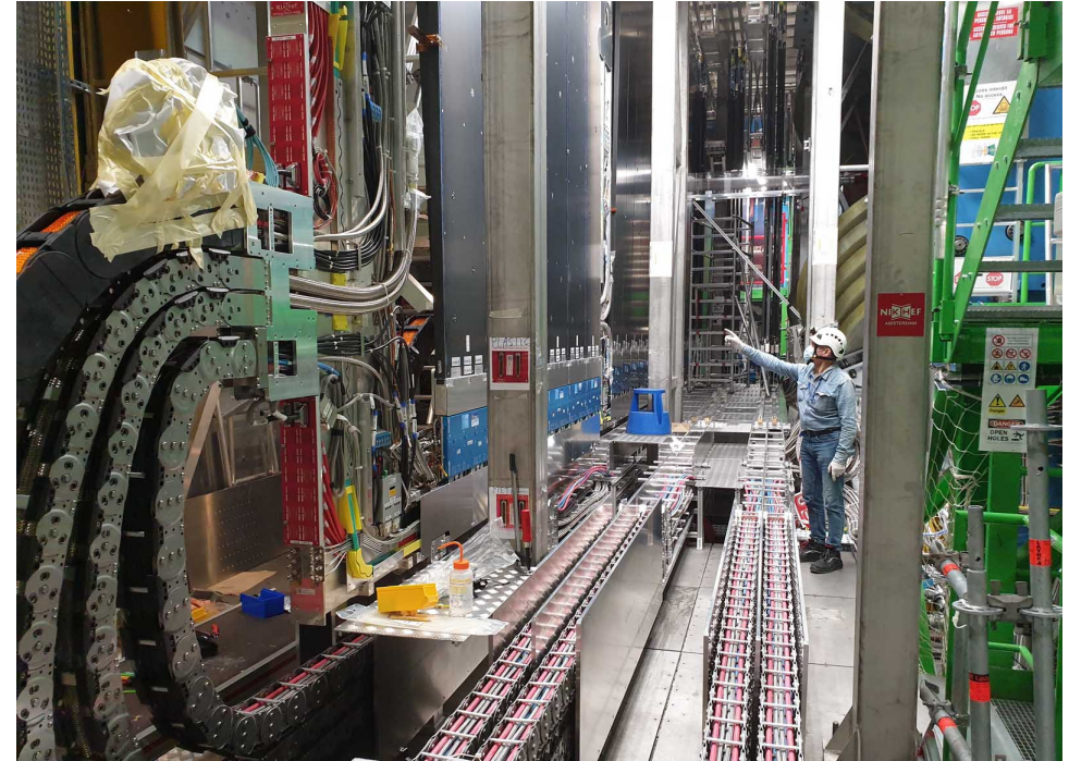
SciFi tracker plane 100 m underground.
