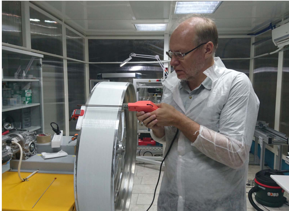
Mat cutting with a hot knife.
