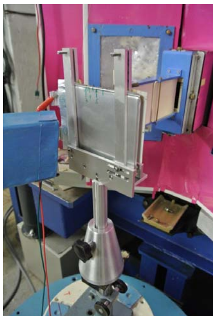
Fig.1. The Li-ion battery mounted on the HRFD instrument for in-situ measurements (on the left). The 10Ah Li-ion cell with contacting electrodes and clips for electric current (on the right).
