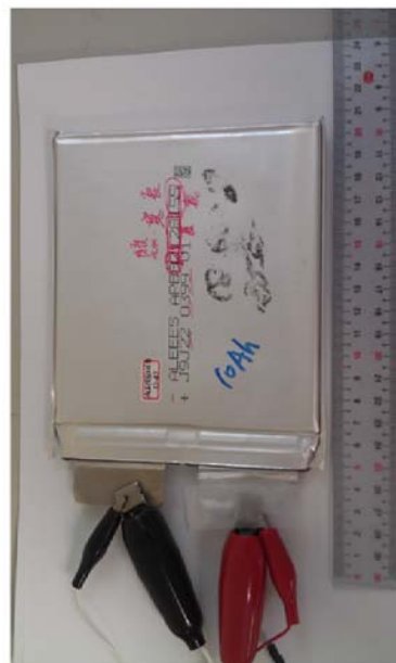
Fig.1. The Li-ion battery mounted on the HRFD instrument for in-situ measurements (on the left). The 10Ah Li-ion cell with contacting electrodes and clips for electric current (on the right).
