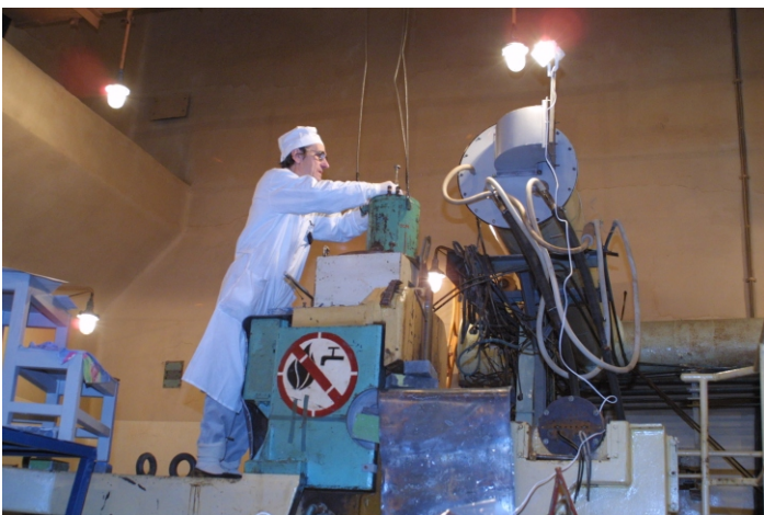
V.D.Denisov extracts a fuel assembly from the core.
