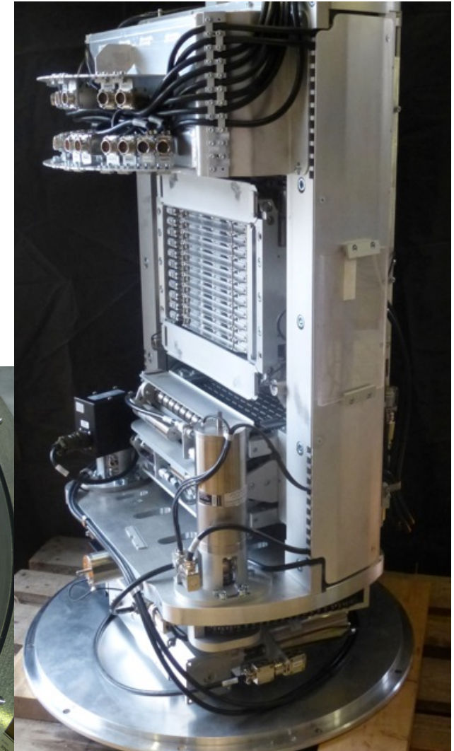
IN8 (2015) monochromator (4x 2D focusing face)
