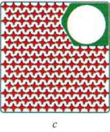
FA sectional view: a – types 1 and 3 (188 fuel elements); b – types 2 and 4 (160 fuel elements); c – type 5 (158 fuel elements)
