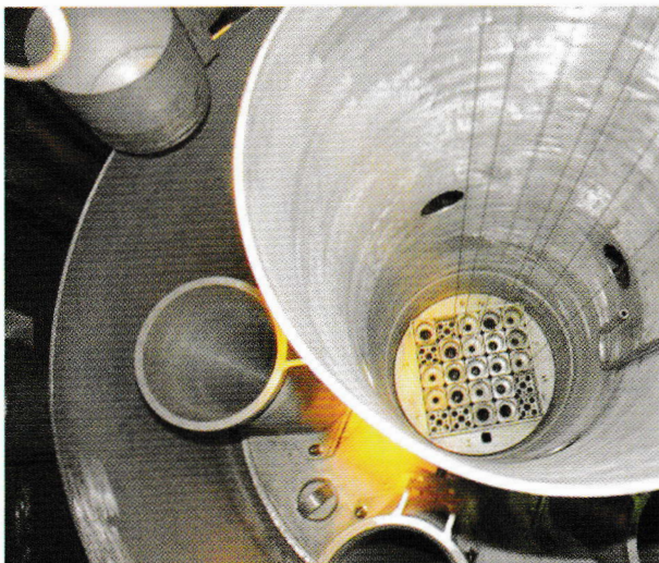
IRV-M2 reactor core and reflector grid
