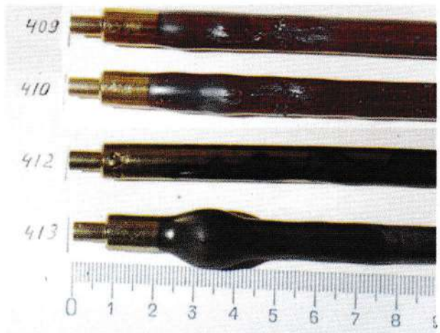
VVER fuel samples after their irradiation in BIGR reactor
