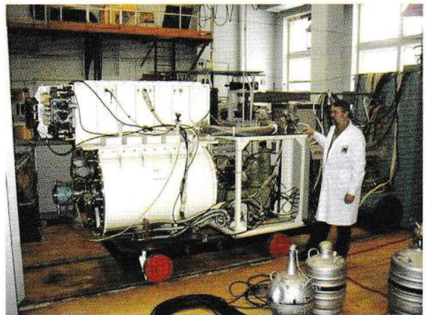
LM-8 eight-channel laser module used in tests of nuclear pumped lasers at BIGR reactor
