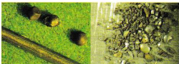
Coated particle fuel before and after its irradiation in BIGR reactor
