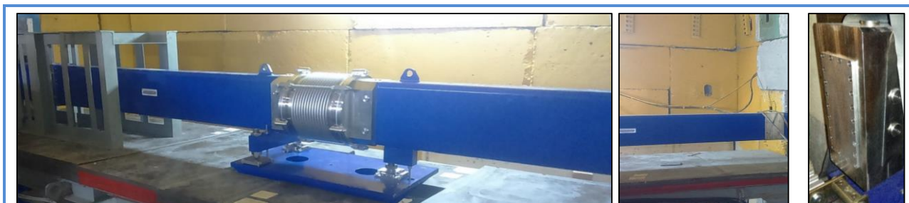
Fig. 4-1. Neutron focusing device with vertical parabolic focusing at the DN-6 diffractometer.
