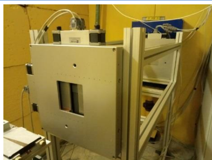
Fig. 4-5. Controllable slit-type apertures for collimating beam directly at the sample position on the GRAINS reflectometer.
