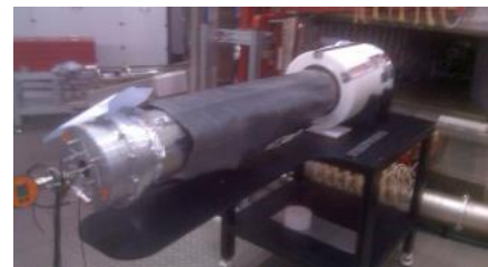
Fig. 5-9. Spectrometer on the basis of a proton recoil telescope at the KSTAR nuclear fusion reactor.
