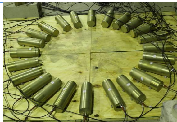
Fig. 3-13. First test geometry for BGO-based detectors.
