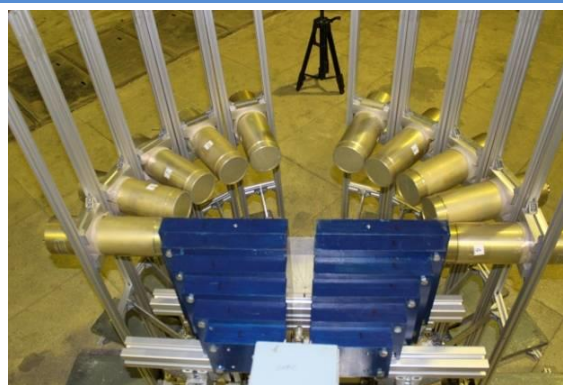
Fig. 3-14. System with 10 detectors, configuration variant "A" – compact geometry with a collimator.
