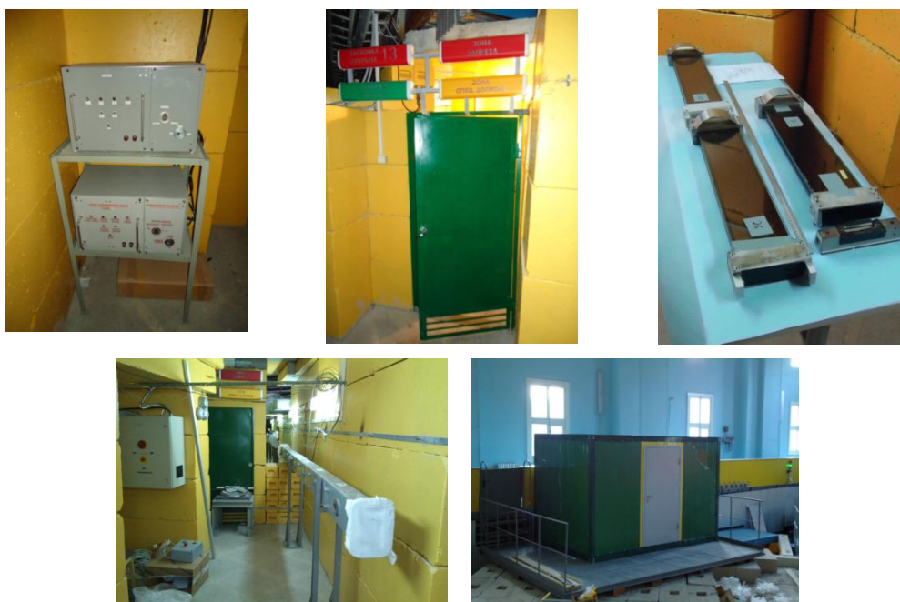
Fig. 22. Fourier-diffractometer FSS on IBR-2 beamline 13 (from top to bottom and from left to right): operational control boxes of a shutter and beam stopper; entrance door to the bunker (beam exit location); glass mirror neutron guide sections before installation in a housing; neutron guide installed in a steel housing and control electronics of the Fourier chopper; experimenter's control cabin mounted on the biological shielding of beamlines № 13-14.
