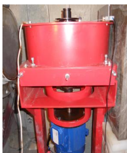
Fig. 23. New drum-type chopper on the REFLEX spectrometer.
