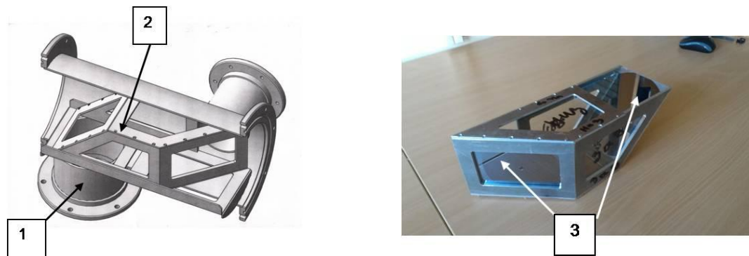
Fig. 23. Sectional view of a spectrum formation unit of the spectrometer (left) and a frame with mirrors (right). 1 – vacuum chamber, 2 – frame with mirrors, 3 – mirrors 1 and 2.
