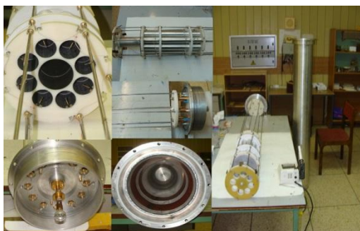
Fig. 19. Electrode system of the new proton telescope (left).
