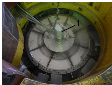
Fig. 14. Photo of a cryocooler cold head (1) in the shaft of the DIN-2PI spectrometer (right).
