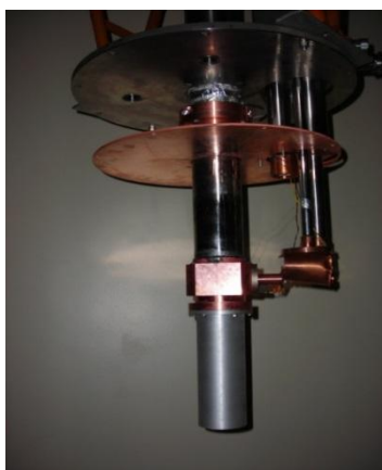
Fig. 71. Shaft cryostat for the NERA-PR spectrometer.
