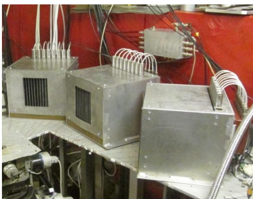
Fig. 66. Small-angle 45^\circ - and 90^\circ -detectors on IBR-2 beamline 6a.
