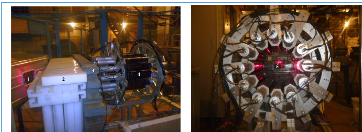
Fig. 29. Experiment to study inelastic scattering of 14-MeV tagged neutrons by ^{12}\text{C} nuclei: 1 - tagged neutron generator ING-27, 2 - polyethylene, 3 - lead, 4 - gamma-detection system "Romashka", 5 - graphite cube.
