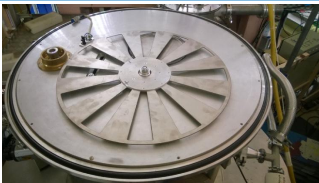
Fig. 53. Multi-slit Fourier-chopper of the Epigraph spectrometer.
