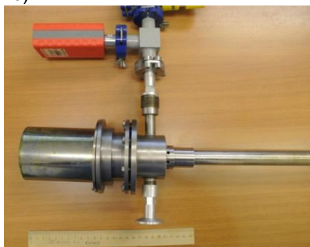
Fig. 16. a) 3D model of a new electrochemical cell for testing electrode materials showing a frame made of corrosion-resistant alloy (green), vanadium current collector plates (yellow), electrode materials (cathode and anode) together with a separator and electrolyte (red), second vanadium current collector, boron nitride and springs (gray), fluoroplastic framing (blue). b) A ready-assembled device for creating special temperature conditions on accumulators.
