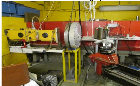
Fig. 46. Ring-shaped helium backscattering detector on the RTD diffractometer.
