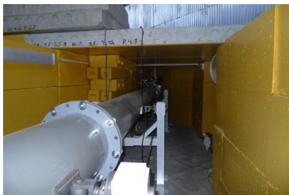
Fig. 15. Vacuum collimation system (a) and CCD-camera-based imaging system (b).
