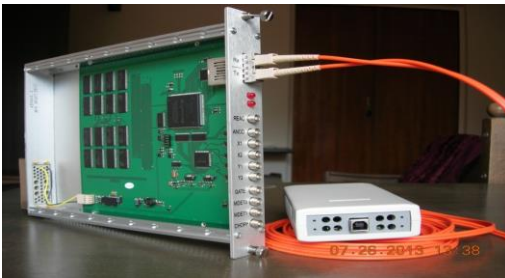
Fig. 55. De-Li-DAQ2 unit for data acquisition and accumulation from PSD.
