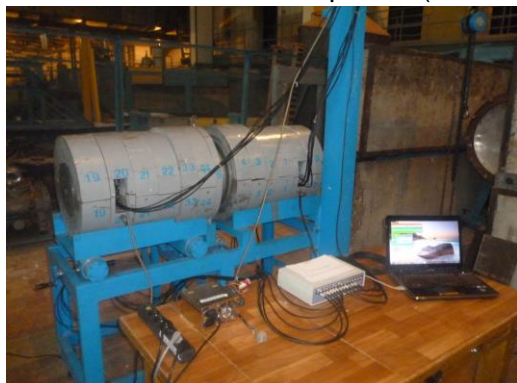
Fig. 19. 12-detector NaI(Tl) gamma-spectrometer system "Romashka" (INRNE-BAS) on beam 4 of the IREN pulsed neutron source.
