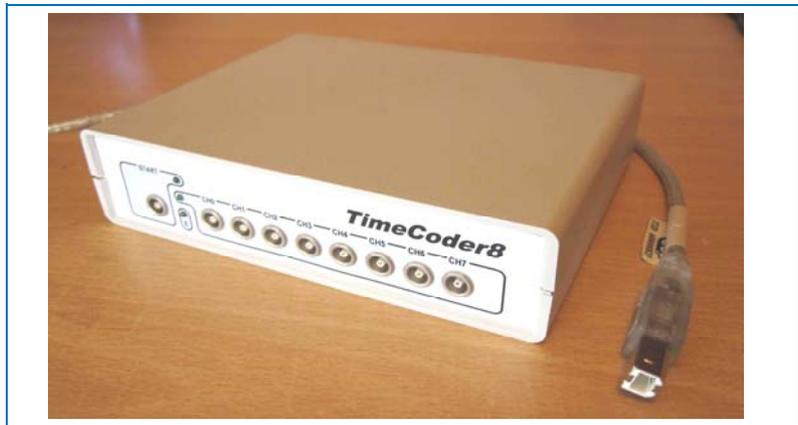
Fig. 21. An overall view of 8-channel time encoder.
