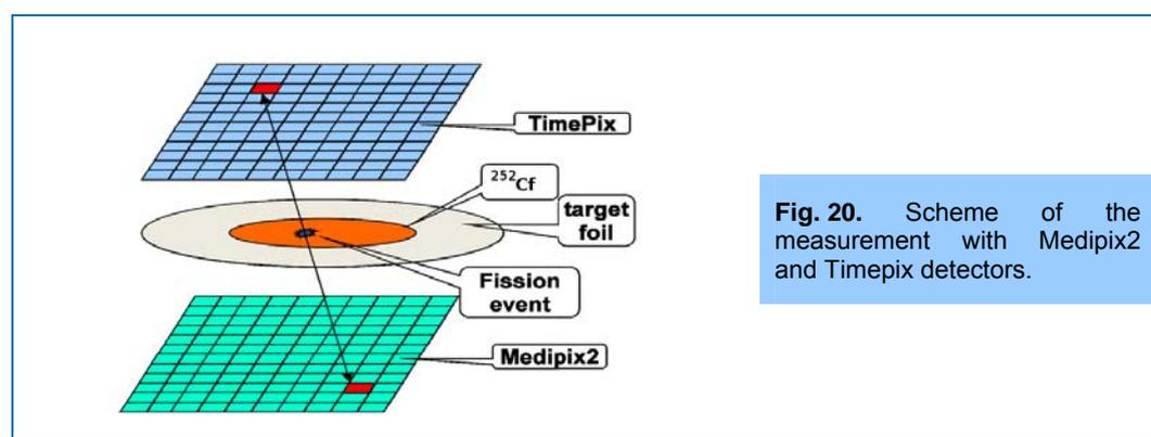
**Fig. 20.** Scheme of the measurement with Medipix2 and Timepix detectors.
