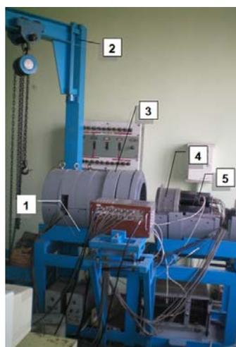
**Fig. 15.** 12-section gamma-spectrometry scintillation system “Romashka-1”: 1 – iron support-holder, 2 – hoisting mechanism, 3 – segmental lead jacket, 4 – assembly of 6 NaI(Tl) scintillation crystals, 5 – photoelectronic multiplier.
