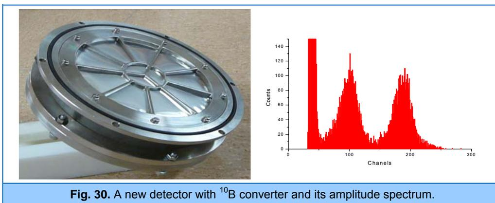
**Fig. 30.** A new detector with  $^{10}\text{B}$  converter and its amplitude spectrum.
