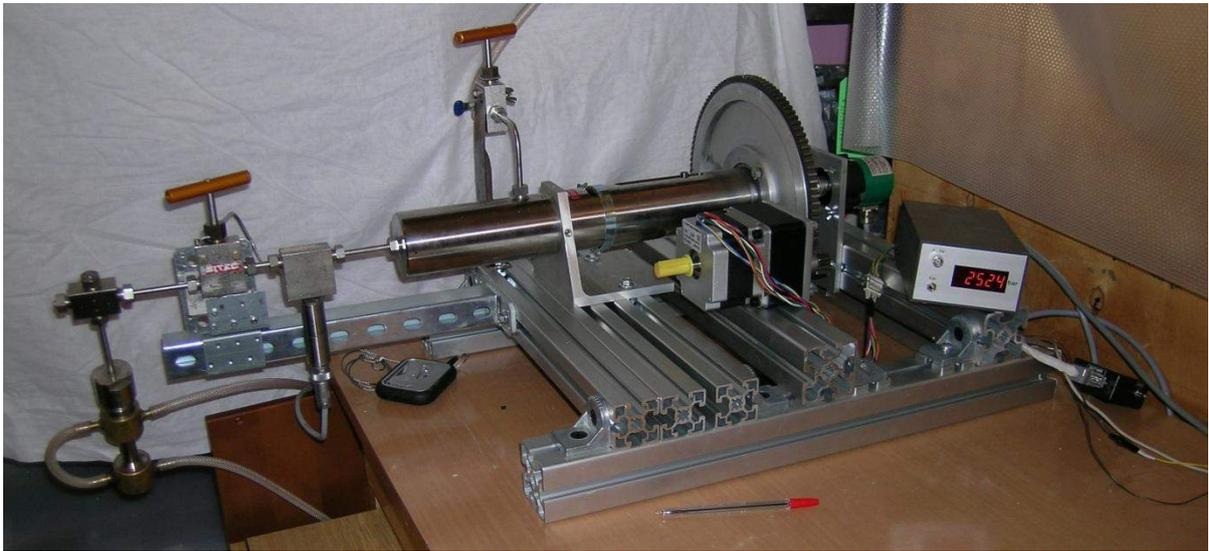
**Fig. 1.** Volumetric high-pressure setup of the YuMO spectrometer, adapted for SANS experiments.
