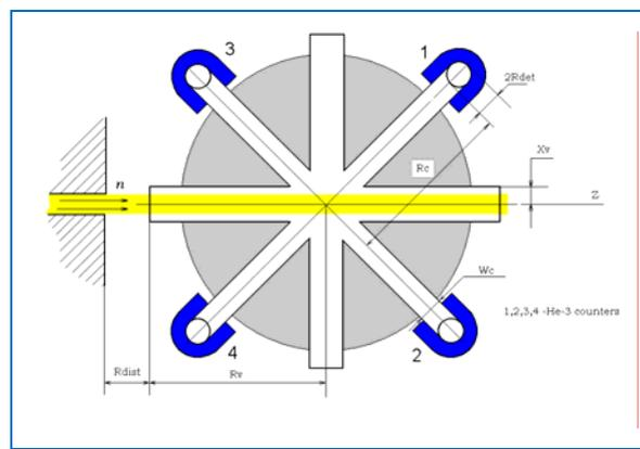
Fig. 22. The layout of the installation for calculation of neutron scattering (top view) 1, 2, 3, 4 – shielded detectors at the ends of collimators fixed on the turn-table.
