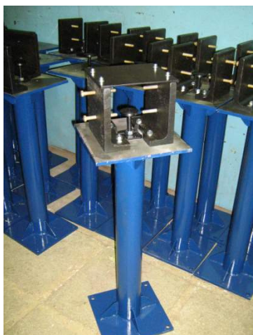
Fig. 2. Beam-positioning support pillars for curved neutron guides
