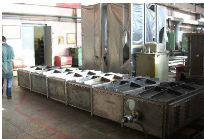
Fig. 1. Splitter housing at a vacuum test site.
