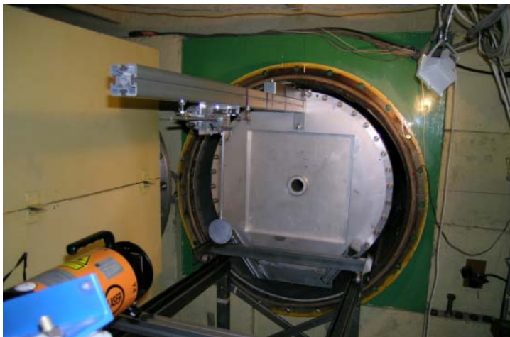
Fig.1. Main view of the PSD with Vn-standard device and the special support for 3-D adjustments to neutron beam inserted in the detectors tube.
