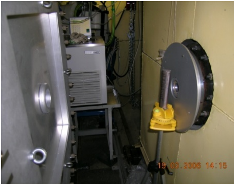
Fig.2. Setup of PSD for backscattering geometry.
