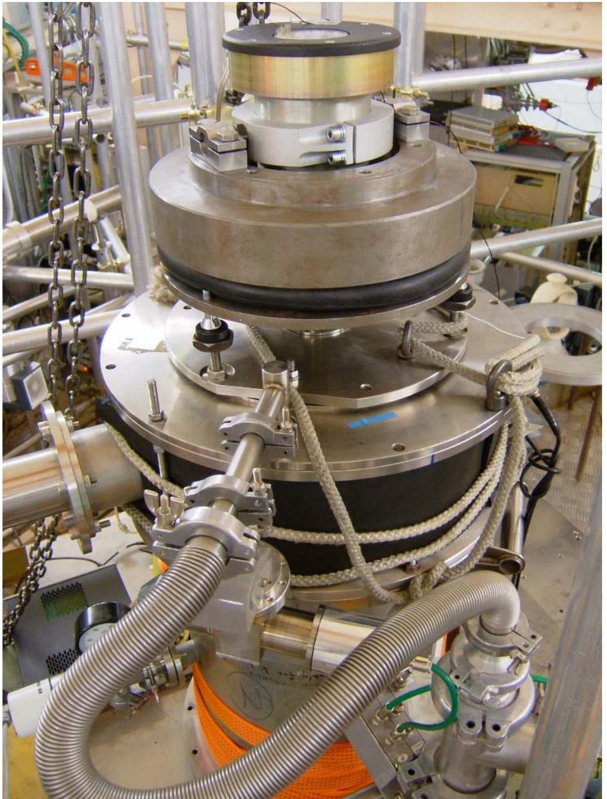
Fig.2. Gravity UCN spectrometer. An electro-magnet driver inducing a harmonical motion to the sample is installed at the upper flange.
