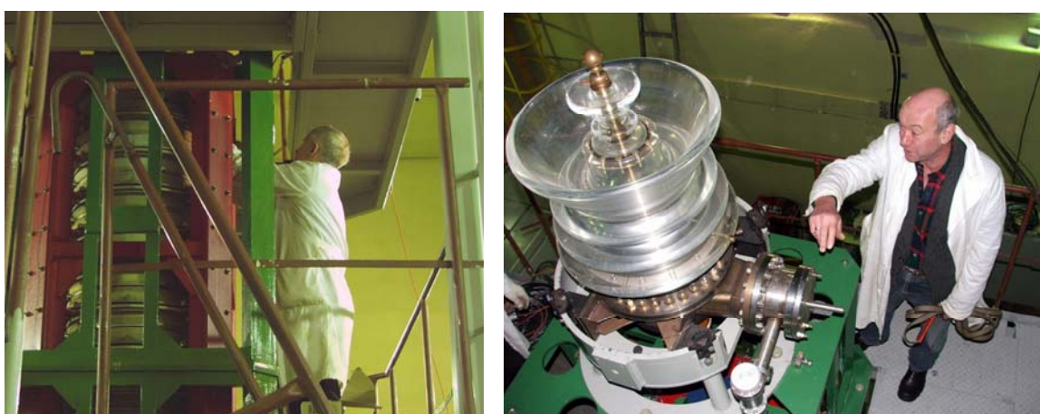
Fig. 2. Mounting of the focusing solenoid (left) and electron gun (right).
