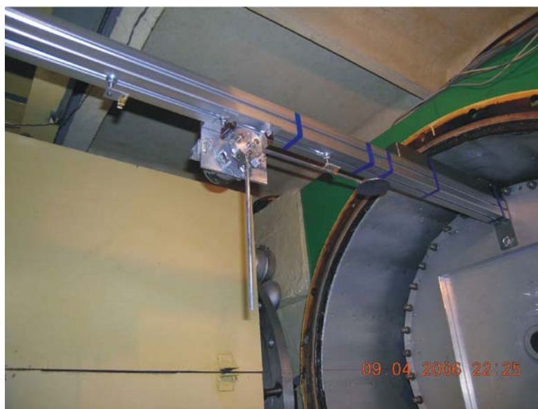
Fig. 5. Device for placing a scatterer into a neutron beam.
