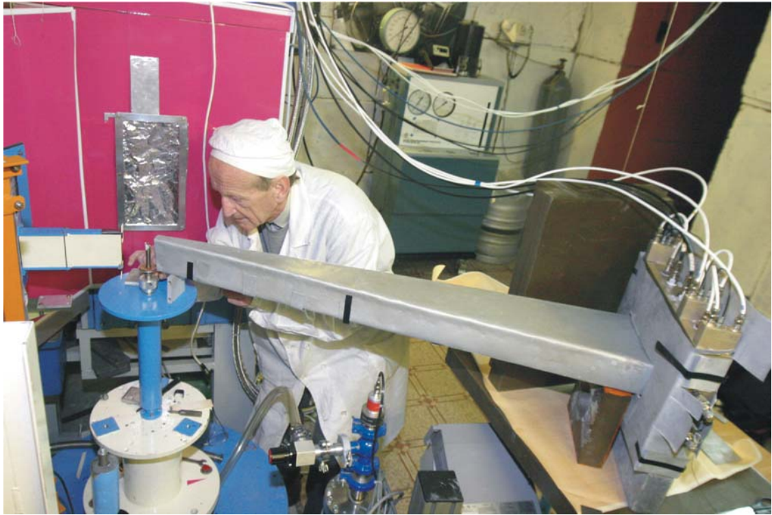
Fig. 6. V.G.Simkin during preparations for tests of 1D position-sensitive detector at HRFD.
