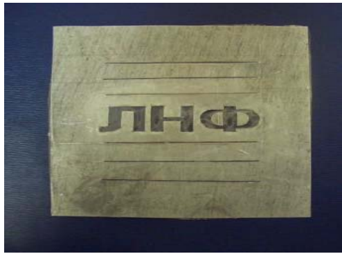
Fig. 5. Exposure measurement using a cadmium mask "ЛНФ". 50 mbar He^3 + 950 mbar CF_4 . Measurement time — 15 min. Voltage across the anode — +3300V.
