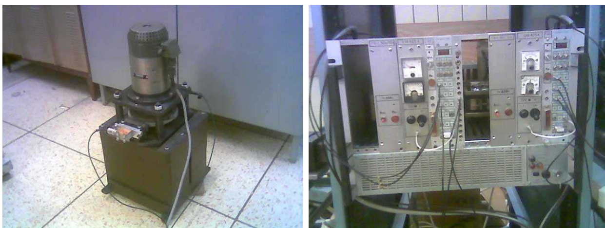
Fig.16. Beam chopper of channel 6b on the basis of direct current electric drive (left) and control system (right).
