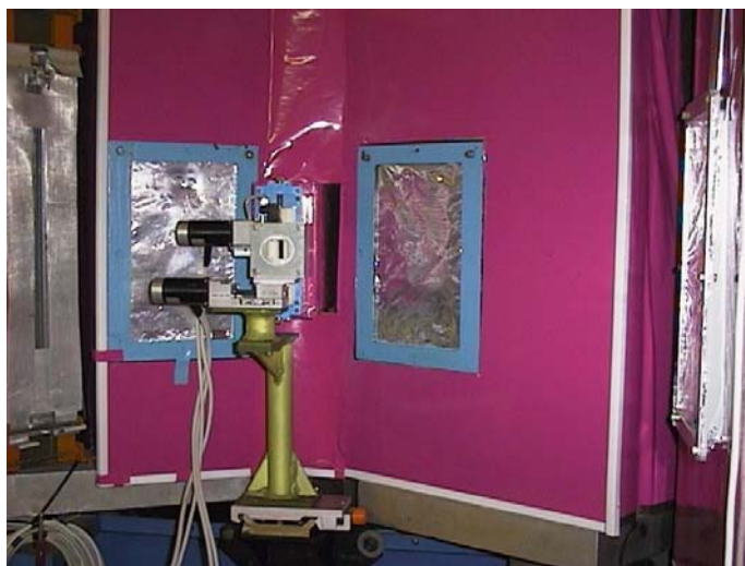
Fig.8. Variable diaphragm with a positioning device.
