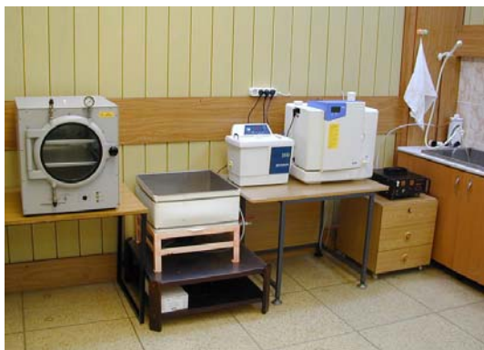
Fig.1. Vacuum furnace, water purifying system and ultrasonic bath.
