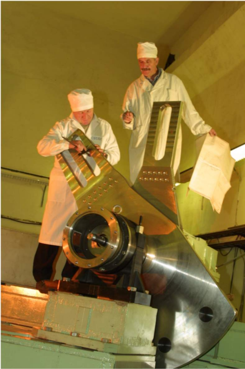
Assembling of a new movable reflector for the IBR-2 reactor on the test-bench
