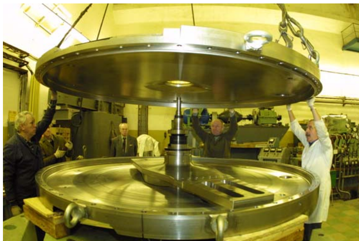
Fig. 2. The IBR-2 reactor personnel at work to assemble the MR-reflector with a jacket on the testing stand in FLNP JINR.
