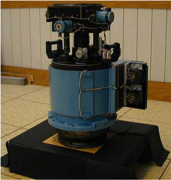
Fig.6. Control system of sample position on the basis of a scanner and platform with a rotary "arm" for placing the detector at the DSD spectrometer
