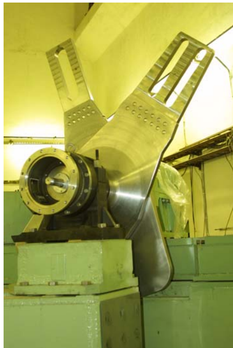
Fig. 1. The new movable reflector MR-3 for the IBR-2 reactor (main and auxiliary reactivity modulators).
