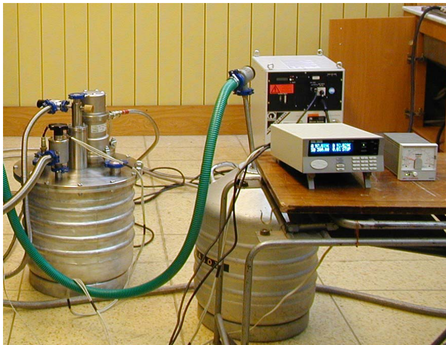
Fig.7. Top loaded closed cycle cryostat on the basis of two-stage cryogenerator CoolPower 100T
