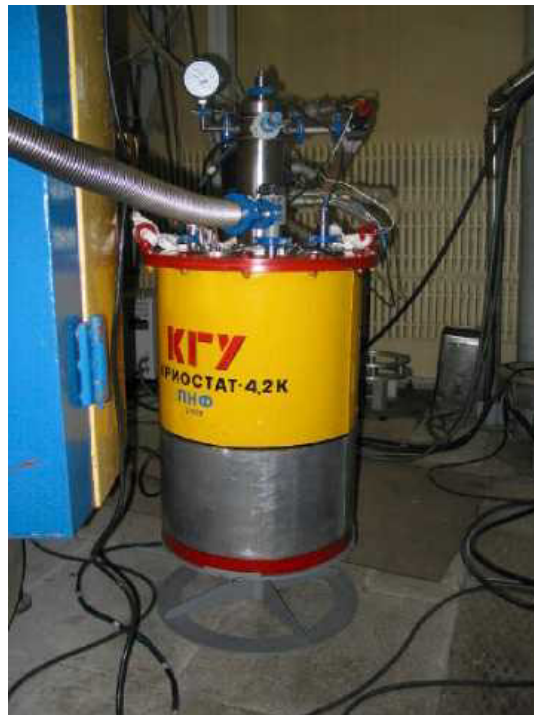
Fig.3. Closed cycle cryostat KFY801 on the basis of two-stage cryogenerator RGD1245.
